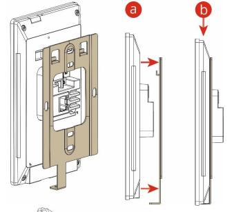
Insert one M2.5 screw below the tablet and secure the tablet to the wall mount bracket.
